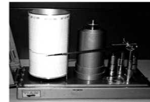
A barograph continually records air pressure through time
