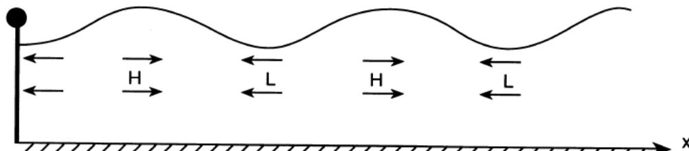
diaphragm at the left end. Labels  $H$  and  $L$  designate centers of high and low perturbation pressure. Arrows show velocity perturbations. (b) The situation  $1/4$  period later than in (a)
