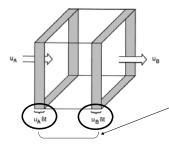
Change in Lagrangian control volume (shown by shading) due to fluid motion parallel to the x axis.
