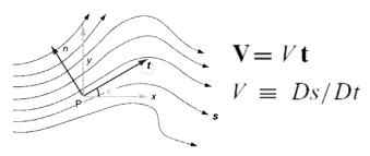
• At any point on a horizontal surface, we can define a pair of a system of natural coordinates (t, n), where t is the length directed downstream along the local streamline, and n is distance directed normal to the streamline and toward the left.
