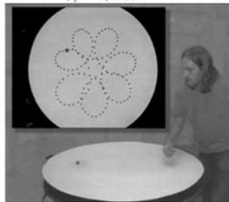
FIGURE 6.13. Studying the trajectories of ball bearings on a rotating paraboloid as described in Durran and Dmonikos (1996). A co-rotating camera views and records the scene from above.
