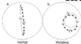
FIGURE 6.14. Trajectory of the puck on the rotating parabolic surface during one rotation period of the table  $2\pi/\Omega$  in (a) the inertial frame, and (b) the rotating frame of reference. The parabola is rotating in an anticlockwise (cyclonic) sense.
