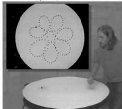
FIGURE 6.13. Studying the trajectories of ball bearings on a rotating paraboloid as described in Durran and Dmonikos (1996). A co-rotating camera views and records the scene from above.
