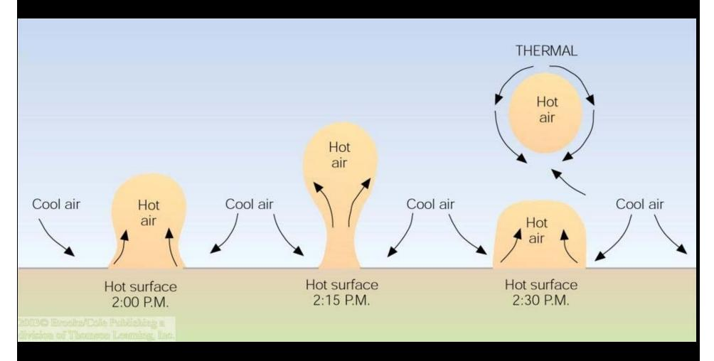
Convection is heat energy moving as a fluid from hotter to cooler areas.
