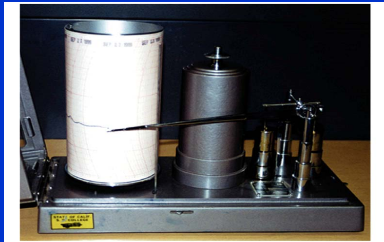
A barograph continually records air pressure through time
