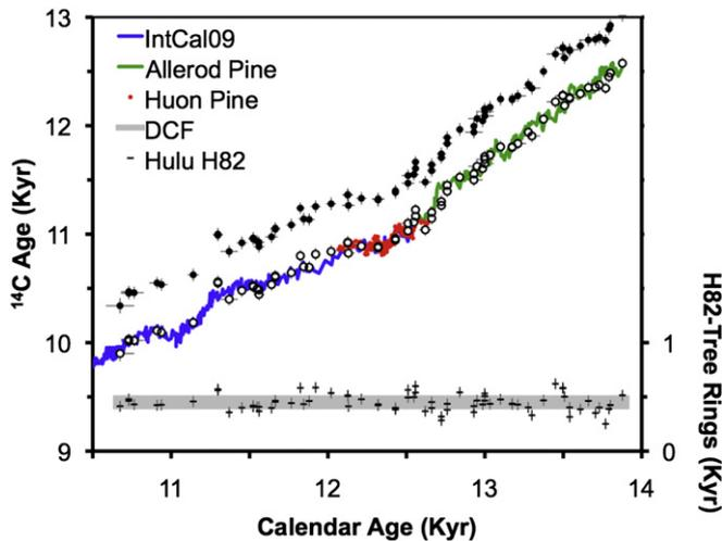
Fig. 3.  $^{14}\text{C}$  measurements on the H82 speleothem plotted with and without DCF correction against an extended tree ring data set: IntCal09 tree rings (Reimer et al., 2009) plus Huon Pine (Hua et al., 2009) and Allerød Pine (Kromer et al., 2004). Tree ring – H82 age differences are shown at the base of the plot, with a grey bar representing the  $\pm 50$  year DCF uncertainty derived from the H82 – IntCal09 comparison.
