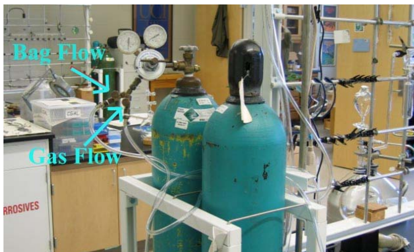
Figure 9. N_2 gas tanks
